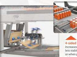
4-sided containment increases efficiency for less stable products or when packaging without trays
